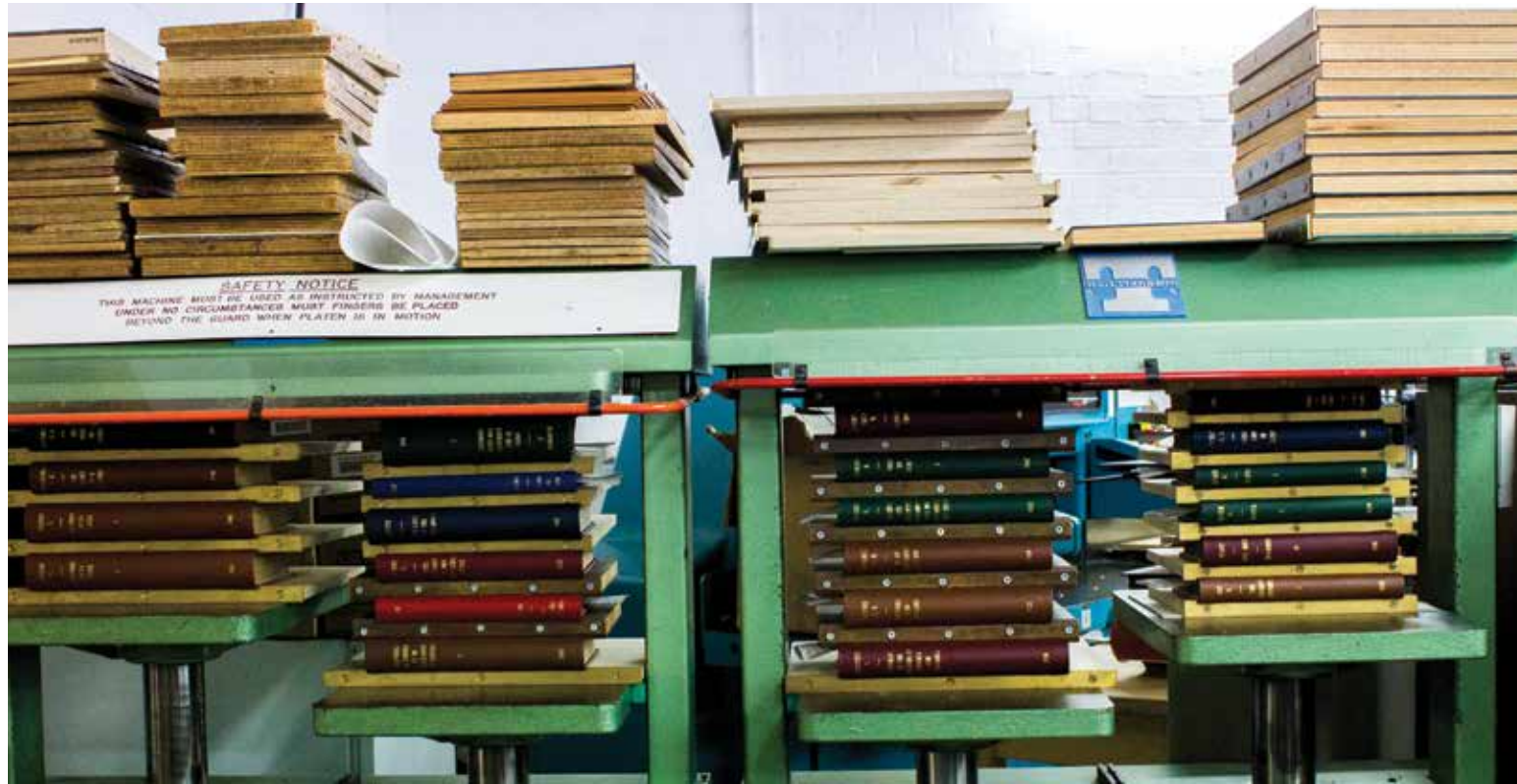
[Clockwise from above] Books for the London Library are pressed after being cased-in; a close-up view of the Swift glue machine, which applies glue to cloth for making book cases - the glue is picked up by two brass rollers as the cloth feeds through it; colourful details; part of Downie Allison Downie's studio in Partick
